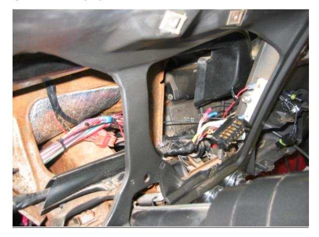
This picture shows the new trailer plug with the jumper currently inserted for testing. I made this connection long enough so the original tach plug would hang down to the bottom of the dash for easy access.
