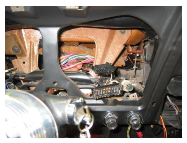
Before reinstalling the terminals into the new plug, be sure to **bend the tab back out** (**bend down**) so that it clicks when the metal terminal is fully pushed into the plug. Give a slight tug on the wire to make sure it won't come back out.
